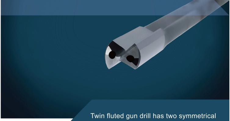
cutting blades and use the same coolant flow system as the brazed single flute gun drill. The coolant oil is supplied through coolant holes in the tool and exit along with the chips in the flutes from the drilled hole.
