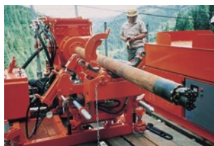
Pipe Roof, Water Service Water Remove, Anchoring It achieves excellent results for drilling of long holes and hard formations using the Down The Hole Hammer. Top-Hammer applications are available.
